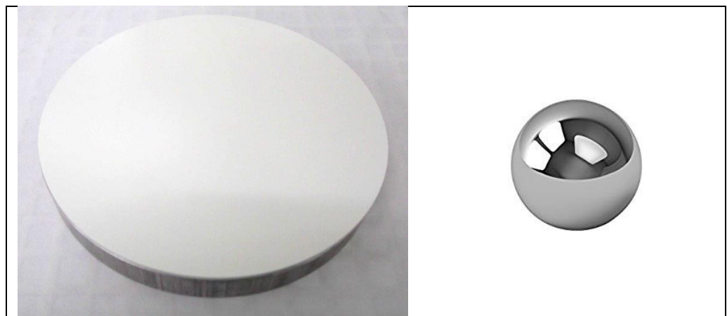
Figure 10 Materials tested – left: Decoclean; – right: stainless steel 1.3541/1.4034
